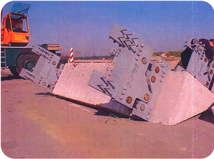
Figure 5 Reinforced concrete cantilever slab fixed on 2 measuring suspensions
